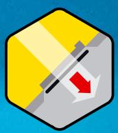
the heat radiates to the interior in the form of long wave infrared radiation which is not transmitted through the glass back to the
