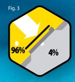
Solar radiation coefficient 'g' informs about the amount of solar energy reaching the glass which penetrates into the room. The higher value of 'g' coefficient, the room heats up
