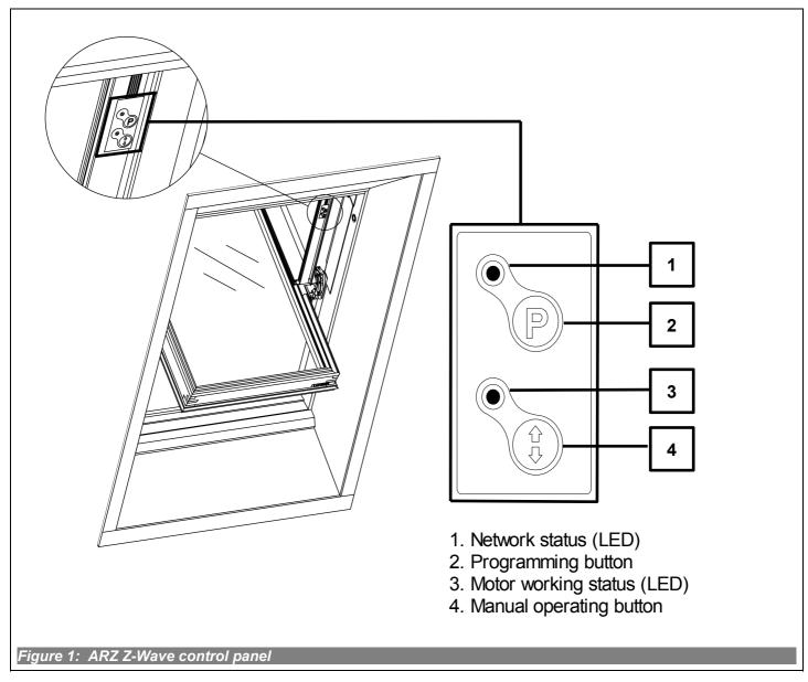
In *Figure 1* there is presented a general view of the available buttons and signaling, situated on the upper right hand guide of the roller shutter.
